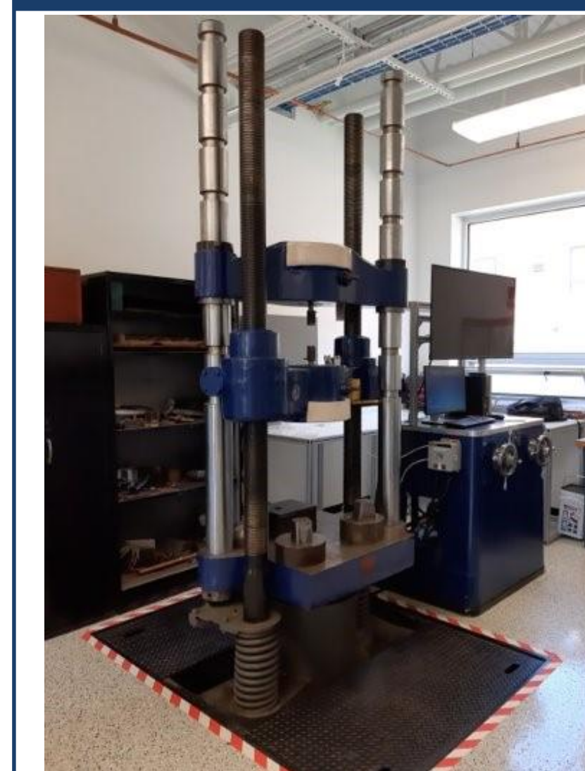
Figure 8: Baldwin Universal Tester pre-modernization.
