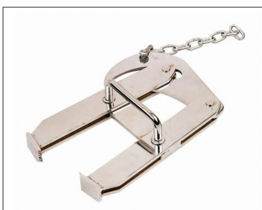
Figure 5: Concept 3 - Pallet Puller
