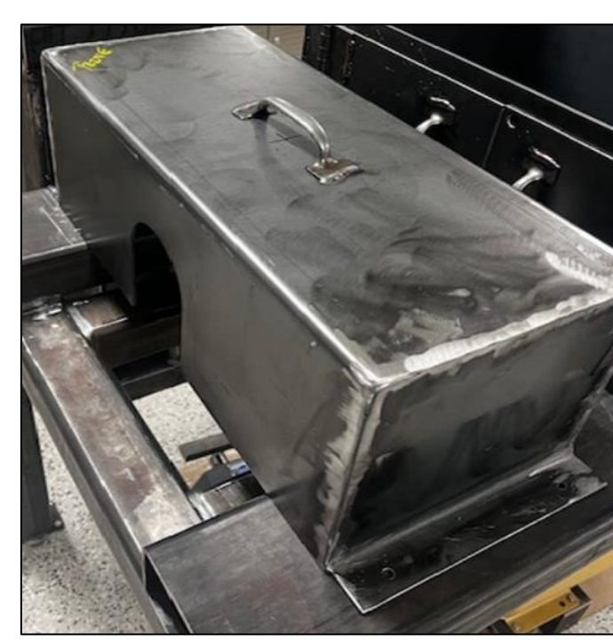
Figure 8: Spindle Box, Conley Welding
