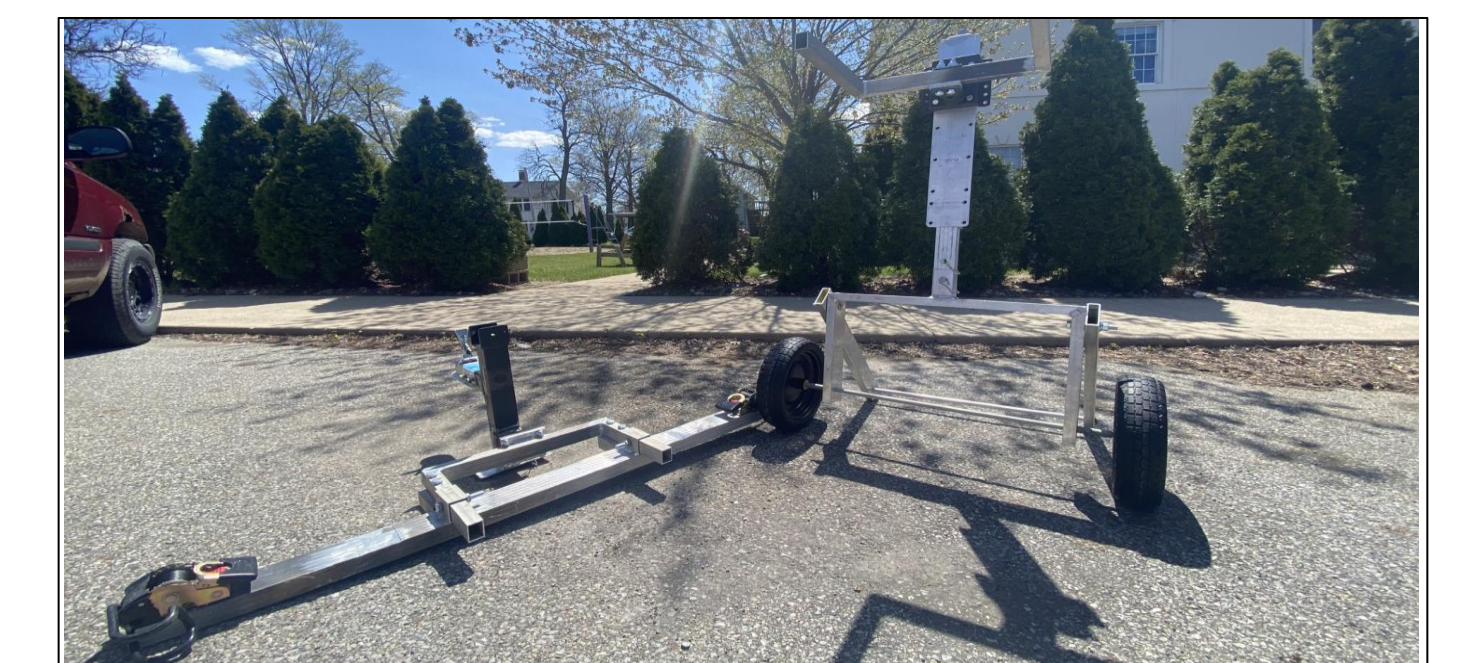
Figures 19: Dock Section Removal Tools
