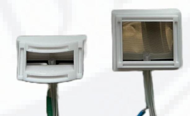
Image 6: 3D printed membrane boxes with integrated sensor & tubing
