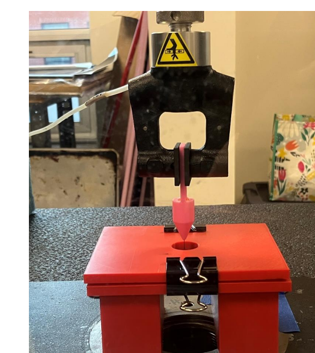
Image 9: Puncture testing set up including Instron machine, samples, and apparatus
