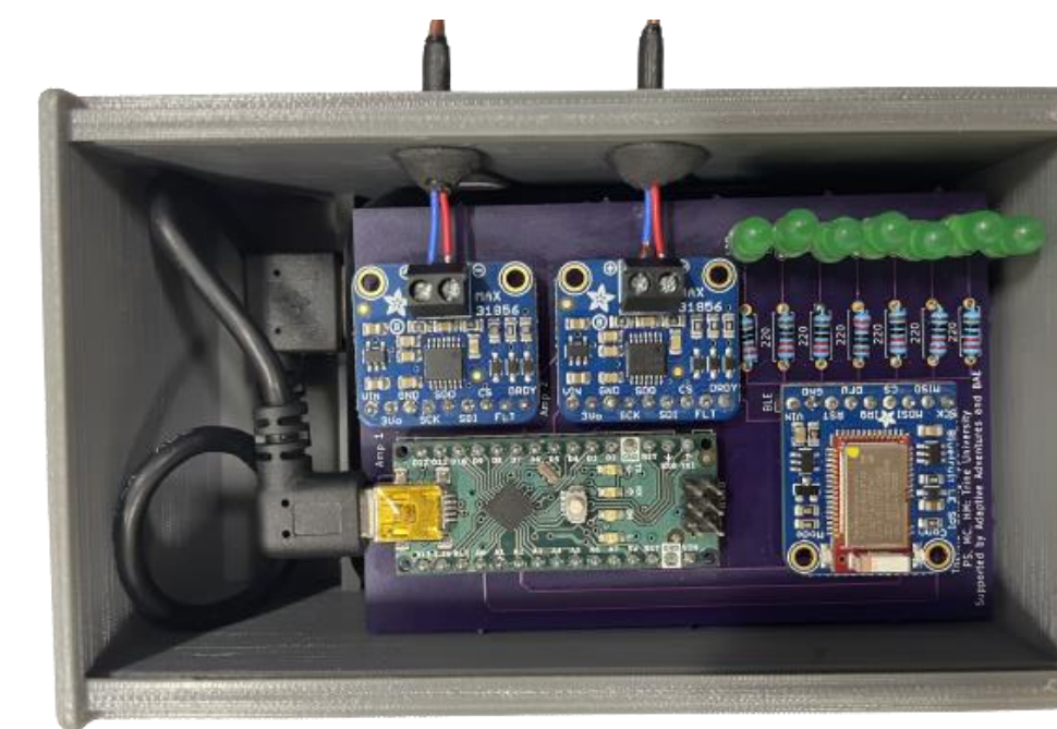
Figure 5: All electronic components are soldered to a custom-printed circuit board (PCB). The Arduino Nano receives power from a power bank battery. The green LEDs draw current to ensure the battery pack remains on.
