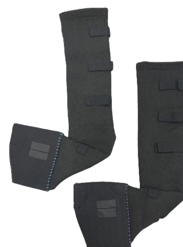
Figure 7: Four custom socks were hand-sewn to ensure adequate fit for various users. Four elastic wire channels line the medial side of the sock to allow for wire securement and wire length customizability. Two sensor slots are located on the dorsal and plantar sides of the sock. Sensors attach to Velcro inside the sock to maintain sensor-skin contact.
