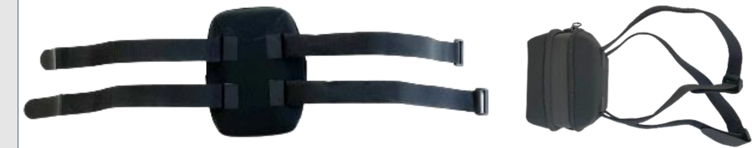
Figure 8: The protective case was developed to provide insulation and shock absorption for the device. Neoprene was selected for superior waterproofing and insulating properties. Slots are located on the back of the protective case to allow for Velcro strap attachment. The temperature sensors exit the protective case through a hole on the bottom. Drop testing was conducted and device remained functional, thus passing the drop test.
