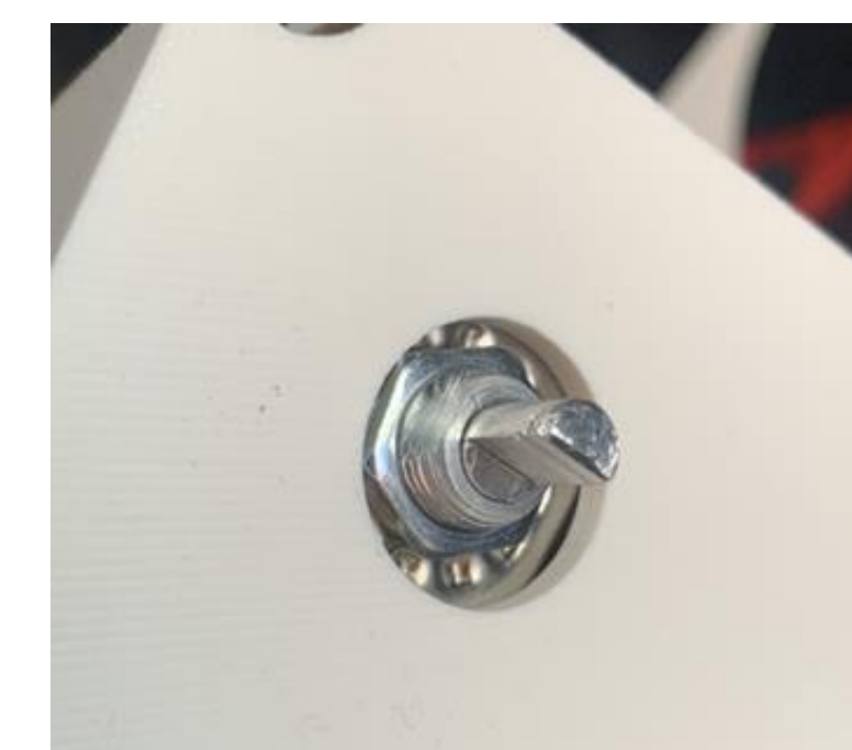
Figure 5: Kill Switch Hole Size Issue
