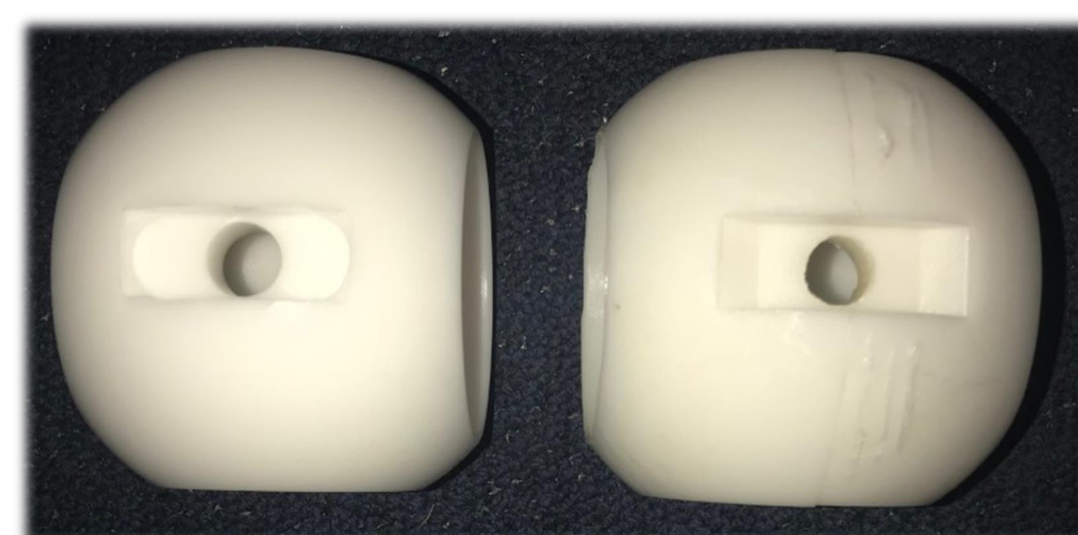
Figure 5: Machined & Unmachined Ball Valve
